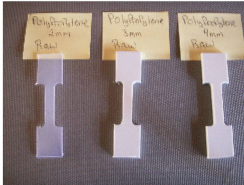
Figure 4 Some samples used in uniaxial tensile testing
